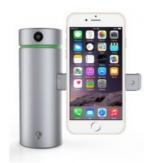
Australian tech start-up Eora 3D recently unveiled a new kind of 3D scanner entirely powered by a modern smartphone. The Eora 3D scanner is completely driven by a smartphone and requires only a one-time calibration. 3D models are rendered inapp, from which users can view, edit, or share or export them in high resolution. The scanner has a range of up to 1 metre and captures in full colour.
