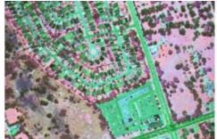
Until now, most commercially available airborne Lidar systems have operated on one single wavelength, reflecting energy from a pulse which is then used for classification or visualisation. New developments have produced the first multispectral Lidar systems, which scan using laser pulses in a number of different wavelengths. Multispectral Lidar data contains valuable information about the
