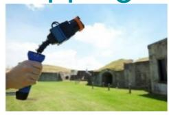
Australian researchers are using the novel mobile laser 3D mapping system called Zebedee to preserve some of the country's oldest and most culturally significant heritage sites. The handheld 3D mapping system is developed by CSIRO and can scan an environment as an operator walks through it.
