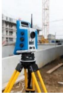
At the Razisse dam on the Dadou River in southwest France, a [Spectra Precision FOCUS 35 robotic total station](#) has just completed monitoring the structural movements that occurred during recent major repairs and improvements to the dam. The FOCUS 35, with its one arc-second accuracy, was chosen to monitor to a half-millimetre accuracy movement of the arch dam abutments during a
