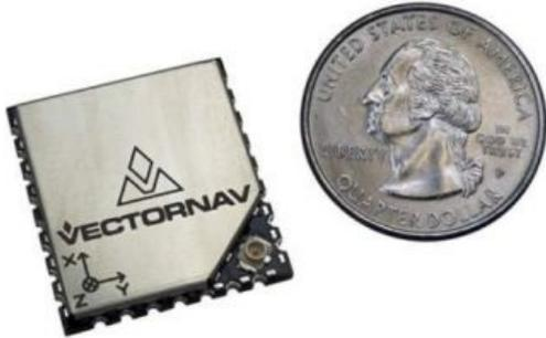
VectorNav Technologies, USA, has presented the VN-200, a high-accuracy GPS-aided Inertial Navigation System (GPS/INS) on a surface-mount chip the size of a postage stamp. Combining an advanced GPS module with MEMS inertial and pressure sensor technology, the patent-pending VN-200 provides a coupled position, velocity and attitude solution that is robust to a wide range of static and dynamic operating conditions.
