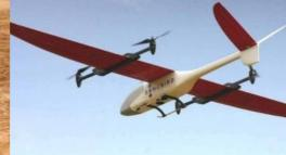
Unmanned airborne systems (UASs) – aircraft which fly without human pilots on board – have soared in popularity as surveying devices. Today they are applied in a wide variety of 2D and 3D mapping, inspection and monitoring tasks. So far there have been two broad categories: fixed wings and multicopters. However, recent advances have led to a third category: the hybrid UAS/UAV, which
