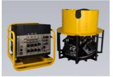
Lead'Air has recently developed a new MIDAS 300P with a Phase One IXU-R 1000 - 100mp nadir camera with a 50mm lens and four Phase One IXU 150 - 50mp oblique cameras with 80mm lenses. The combination of these two camera models creates a high-quality, medium-format imaging system for combination oblique/vertical image capture.
