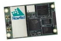
NovAtel, a leading OEM provider of high-precision GNSS positioning products, announced the release of the OEM617D receiver at AUVSI's Unmanned Systems 2014. The OEM617D is a compact, dual-antenna, dual-frequency, single-card receiver offering NovAtel's leading ALIGN heading functionality and its RT-2 Real Time Kinematic (RTK) GNSS positioning technology, in dynamic and static environments.
