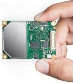
Topcon Europe Positioning, The Netherlands, has announced a light, ultra-compact dual-frequency positioning engine, the B110 GNSS receiver board for OEM applications. The B110 is the first GNSS board with Topcon's Vanguard ASIC, supporting 226 universal channels for GPS, GLONASS and Galileo tracking and scalable positioning from sub-metre DGPS to sub-centimetre RTK.
