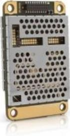
Satel, a Finnish manufacturer of radio data transmission systems, aims to set a new milestone with the launch of the new Satellite TR4. This compact UHF transceiver with transmitting power of 1,000mW is compatible with the protocols of Pacific Crest, Trimble and Satel. The type certifications in all important regions of the world make the Satellite TR4 very suitable for integration in end devices that are intended for international use.
