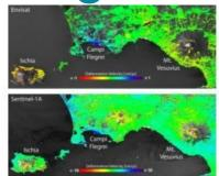
Thanks to frequent observations from the year-old Sentinel-1A radar satellite, scientists are improving the remote sensing technique to map ground deformation and hence opening new doors for earthquake and volcano monitoring. By comparing data from past satellite radar missions – ERS and Envisat – with those obtained from the current Sentinel-1A, researchers of Italv's
