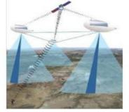
Unmanned Aerial Vehicles (UAVs) flying for months or years above the Jet Stream will form a new communication and sensing infrastructure. National security payloads will emphasise sensors like cameras or signals intelligence receivers plus robust radio relay. Commercial payloads will emphasise very high data rate communications with some sensors like visible light and multi-spectral cameras.
