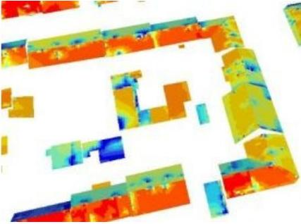
New software paves the way for the use of renewable energies on roof areas. Tridicon SOLAR generates a planning instrument automatically. Part of the challenge of renewables is the search for new locations where solar panels using photovoltaics technology or solar thermal power will be efficient. Municipalities, energy suppliers, investors and citizens need a planning instrument that visualises the solar potential of roof areas taking into account exposition, slope and shadowing.
