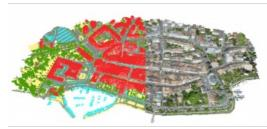
Pix4Dmapper is an industrial-standard photogrammetry software package that provides accurate 3D reconstruction from overlapping images. Along with the expanding drone market, people are keen to explore new solutions to replace or to complete traditional technologies. Point cloud classification, an iconic feature for Lidar point cloud, is now also being considered by drone surveying professionals.
