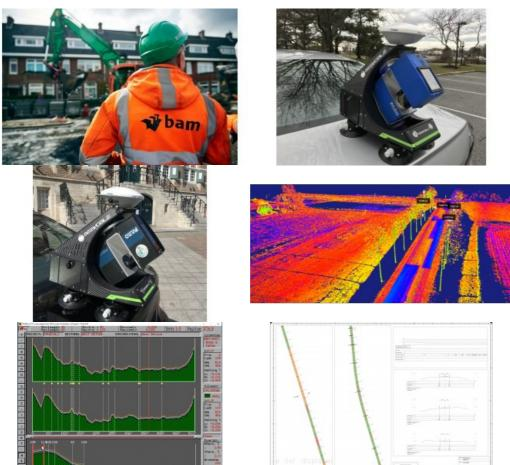
BAM Infra recorded 3D road models using a Faro terrestrial laser scanner with the innovative BeeMobile mobile mapping system at various locations across the Netherlands in 2020.
