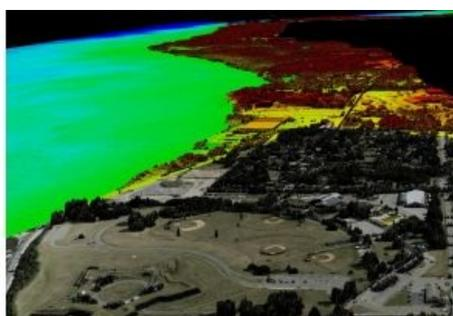
“Think big for coastal mapping” is the foremost advice that Don Ventura of [Teledyne Geospatial](#) would impress upon agencies interested in bathymetric Lidar. “It’s a matter of efficiency of scale.” Airborne bathymetric Lidar can actually be more efficient and cost less per square kilometre than acoustic methods in nearshore, optically-suitable waters. Data collection with airborne bathymetric Lidar
