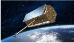
Designed to operate for five years, Airbus's Synthetic Aperture Radar (SAR) satellite TerraSAR-X has achieved ten years of flawless operations in orbit providing highresolution radar images in all weather conditions, 24 hours a day. Developed and constructed by Airbus Defence and Space teams from Friedrichshafen for the German Aerospace Centre (DLR), the satellite orbits at a height of 514km and provides radar imagery to a wide variety of scientific and commercial users.
