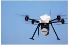
AltiGator and YellowScan have launched an ultra-light weight Lidar UAS combo allowing centimetric UAV surveys in urban areas, in accordance with most regulations. The YellowScan Surveyor ultra-light stand-alone Lidar system is embedded on the OnyxStar XENA multirotor UAV, which is the last generation professional UAV designed by Altigator.
