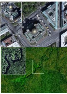
The <u>A3 Edge digital mapping system</u> is a sweeping camera system able to produce high-resolution and accurate imagery from high flight altitudes and hence to conduct surveys quickly and efficiently. The system is suited for capturing urban areas as well as sparsely populated landmasses. In 2014 it was used for two projects in Russia: 3D mapping of Saint Petersburg and mapping of boreal forests.
