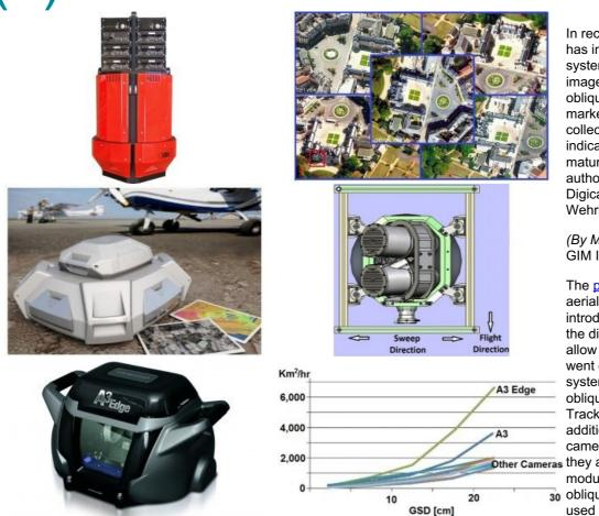
In recent years, aerial photogrammetry has increasingly been using camera systems which capture nadir and oblique images at the same time. The number of oblique systems on offer in the marketplace for airborne geodata collection is growing steadily – a strong indicator that the technology is rapidly maturing. In this follow-up article, the author highlights oblique systems from Digicam, Dimac, Icaros, VisionMap and Wehrli.
