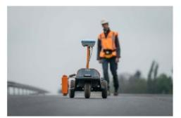
using mobile and terrestrial mapping equipment which produces both a point cloud and panoramic photographs. All these efforts contribute to deliverables such as the Common Data Environment (CDE), building information modelling (BIM) datasets and digital twins.
