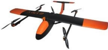
G170-V, a vertical take-off and landing (VTOL) fixed-wing unmanned aerial vehicle (UAV), is the latest UAV German-based GerMAP has added to the remote sensing and aerial mapping market. G170-V ideally combines the easiness of manual or automatic vertical take-off and landing procedures of multicopters with the area coverage efficiency of aeroplanes.
