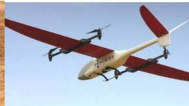
Unmanned airborne systems (UASs) – aircraft which fly without human pilots on board – have soared in popularity as surveying devices. Today they are applied in a wide variety of 2D and 3D mapping, inspection and monitoring tasks. So far there have been two broad categories: fixed wings and multicopters.
