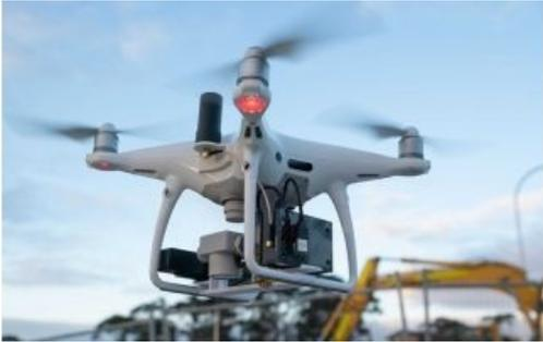
Klau Geomatics, an Australian geospatial innovation company, has announced the KlauPPK enabled 'DJI Phantom4Pro Surveyor', a small drone for accurate surveying. This premium solution brings survey grade PPK direct geo-referencing accuracy to the less than 2kg UAV class, offering a capable, accessible entry point for surveyors to embrace UAV technology.
