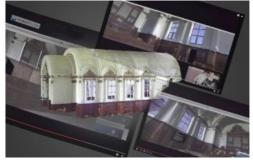
Theatrework UK, a Scottish production company, is using laser scanners and 3D computer modelling technology to help visualise stage productions. Using Pointfuse software, laser scanned data – point clouds – are processed in minutes to create highly accurate 3D models. These models allow production designers to conceptualise ideas within the venue scans and technical staff to visualise touring productions at different venues.
