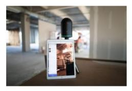
Leica Geosystems has announced that its <u>BLK360</u> miniaturised 3D imaging laser scanner is now available for reservation within Europe, for delivery in summer. The laser scanner simplifies the collection of as-built reality capture data for work in architecture, design, construction and engineering, among other vertical markets.
