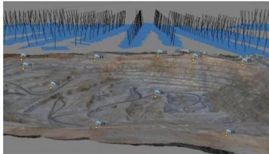
In early May 2018, the Czech company UpVision used an unmanned aerial vehicle (UAV) to map a copper mine in Mongolia – the largest in Asia – as part of an ongoing Czech geological expedition at the site. More than 10 square kilometres of the mine and its surroundings were mapped using the MAVinci Sirius unmanned aircraft.
