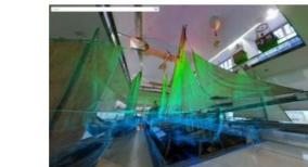
Few museums, shopping centres, airports and other indoor spaces have been mapped, although the demand for detailed 3D models of such spaces is accelerating rapidly. Here, the authors present a trolley-based system equipped with laser scanners, cameras and advanced software aimed at creating, visualising, navigating through and exploring detailed and accurate 3D models of indoor spaces.
