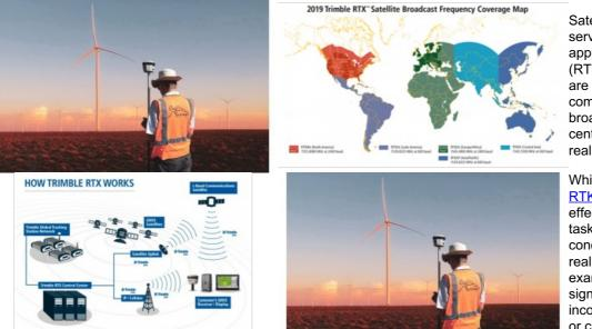
Satellite-delivered GNSS correction services can be used in many real-time applications where real-time kinematic (RTK) and virtual reference stations (VRS) are not available. In areas without regular communication systems, satellitebroadcast PPP corrections can deliver centimetre-level positioning worldwide in real time.
