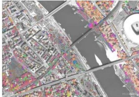
Millions of trees in an area spanning over 500 square kilometres are being monitored in Warsaw, Poland. This unprecedented mapping project of the urban green environment, which is based on a unique multisensor photogrammetric platform, will result in the Tree Crown Map: an advanced map of individual trees, including recognition of nearly 50 taxa, geometry of their canopies and their
