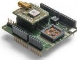
Xsens has expanded its MTi product portfolio by introducing the [MTi-7](#), a miniature inertial navigation system (INS) module which uses input from an external global navigation satellite system (GNSS) receiver to provide an accurate, real-time position, velocity and orientation data stream.
