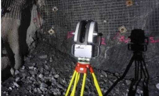
Maptek has launched its new I-Site SR3 600m range laser scanner, developed to become the mine measurement standard for underground operations, both for general underground survey and detailed geological face mapping.
