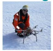
Engineers on board the Alfred Wegener Institute's research icebreaker *Polarstern* have programmed an unmanned autonomous vehicle (UAV), allowing it to navigate despite the deviations produced by the Earth's magnetic field near the North Pole. The researchers recently celebrated the multicopter's first successful autonomous flight and landing on an ice floe.
