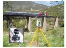
Robotic theodolites, the new generation of the well-known surveying theodolite, are used to measure deflections in short-span bridges with millimetre accuracy. This permits the coming true of an old dream for engineers: to be in a position not only to predict, but to measure the excitation of engineering structures due to dynamic loads such as wind and traffic, and hence evaluate their structural health.
