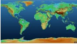
The German space agency (DLR) has released a 3D height map of Earth. Built from images acquired by two radar satellites (TerraSAR-X and TanDEM-X), it traces the variations in height across all land surfaces - an area totalling more than 148 million sq km. DLR is making the map free and open, enabling any scientist to download and use it. The map was made by the satellites sending down microwave pulses to the surface of the planet and then time how long the signals take to bounce back.
