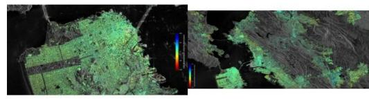
The Sentinel-1 satellites have shown that the Millennium Tower skyscraper in the centre of San Francisco, USA, is sinking by a few centimetres a year. Studying the city is helping scientists to improve the monitoring of urban ground movements, particularly for subsidence hotspots in Europe.
