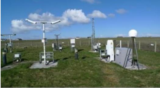
There are more than five billion satnav devices on Earth. Along with smartphones and mobile receivers, this figure includes networks of continuously operating receiver stations (CORS) used to improve accuracy. A European Space Agency-led project will harness these networks to provide an ongoing overview of satnav performance from the global to national and regional scale.
