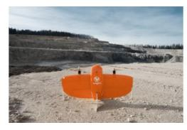
Switzerland-based start-up Wingtra has developed a vertical-take-off-and-landing (VTOL) unmanned aerial vehicle (UAV or 'drone') that rises straight up, tilts and flies off like an aeroplane. The WingtraOne is a broad-coverage drone that is used particularly in the surveying, construction and precision agriculture industries and
