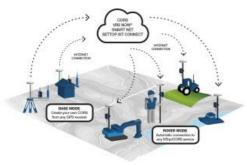
Settop Survey, based in Barcelona, Spain, has launched and released the innovative Settop CellXtrem modem, which is compatible with all GPS manufacturer receivers. The Settop CellXtrem opens the possibility for users to transmit Real-Time Kinematic (RTK) corrections from a base station via internet in a simple, user-friendly way, just using a SIM card without any need of a static IP.
