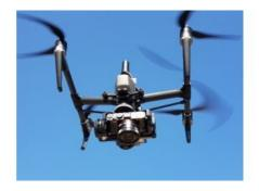
With the end of the DJI X4s camera, drone operators have been looking for a quality mapping camera solution for the Inspire 2 and M200/M210/M210V2 drones. Klau Geomatics has released a Sony camera/PPK payload to offer better results from these drones. This enables more effective and accurate mapping and inspection using superior-quality, plug-and-play camera payloads with precise 3D positioning accuracy.
