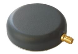
Tallysman has introduced the TW2920 antenna for simultaneous reception of L-band correction signals and all of the upper band GNSS signals including GPS L1, GLONASS G1, Galileo E1, and BeiDou B1. The TW2920 1dB bandwidth covers 1525MHz to 1559MHz for the L band down-link and 1559MHz to 1610MHz for the upper band GNSS.
