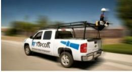
Topcon has released its latest positioning solution: IP-S2. This system is a fully integrated positioning solution which provides high rate, high accuracy, real-time or post processed position and orientation information for land based vehicles. IP-S2 incorporates a top of the line, survey grade GNSS receiver with an inertial measurement unit and vehicle odometers to provide more accurate and robust positioning information than GNSS alone.
