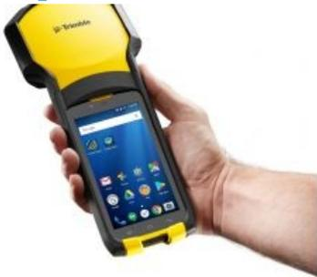
Trimble has announced a new high-performance field computer for its Mapping and Geographic Information Systems (GIS) portfolio – the Trimble TDC150 handheld. Designed for GIS data collection, inspection and management activities, the TDC150 provides users a rugged solution that has the flexibility of a handheld, a modern interface with open Android operating system, and scalable high-accuracy positioning for professional field workflows.
