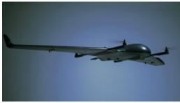
Vertical Technologies has released its DeltaQuad series of autonomous VTOL UAVs. This hybrid vertical-take-off fixed-wing UAV can stream telemetry and video over the cellular network <u>using VPN</u>, and boasts a 1kg payload capacity, flight time of 2 hours 45 minutes and 150km range.
