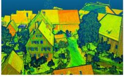
Lidar mapping based on unmanned aerial vehicles (UAVs or 'drones') can generally be thought of as a close-range version of manned airborne laser scanning. In brief, lower mobilization costs and much higher spatial resolution are allowing new Lidar mapping use cases in several disciplines, such as forestry, bathymetry, archaeology, infrastructure mapping, hazard management and so on.
