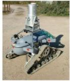
3D Laser Mapping (United Kingdom) has developed a laser-scanning robot to provide an electronic eye in dangerous and in-hospitable environments. Using laser scanning units combined with wireless communications and advanced robotic technology the 3D-R1 allows a 3D map of the surrounding area to be created.
