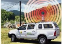
3D Laser Mapping (United Kingdom) has launched a new mobile mapping system specifically designed to capture highly accurate 3D measurements of overhead telecom networks.
