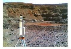
3D Laser Mapping (United Kingdom) is helping Kumba Iron Ore to improve the safety of iron ore extraction in South Africa. 3D Laser Mapping has supplied and installed a Riegl LMS Z420i laser scanner, the first scanner of its type in South Africa.
