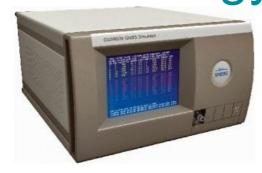
GRACE has taken delivery of a Spirent GSS8000 hardware simulation system, replacing an earlier GSS7700 GPS system. The new system, one of the first to be delivered in the UK, consists of a two chassis, 16 channel GSS8000 system controlled by Spirent's SimGEN software that can simulate current and future GPS signals, including L1, L2 and L5 signals and Galileo E1, E5 and E6 signals as well as WAAS and EGNOS Space Based Augmentation System signals.
