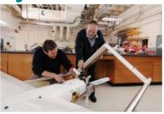
American researchers at the Georgia Tech Research Institute (GTRI) are currently working on the development of an airborne testing capability for sensors, communications devices and other airborne payloads. This aerial test bed is called the GTRI Airborne Unmanned Sensor System (GAUSS). GAUSS is based on an unmanned aerial vehicle (UAV) made by Griffon Aerospace and modified by GTRI.
